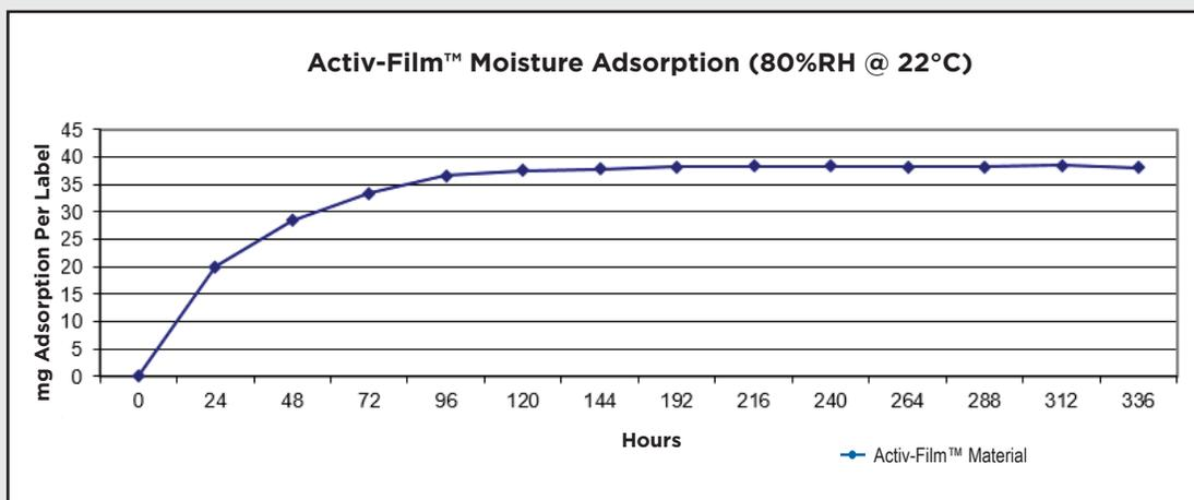
Figure 1: Moisture adsorption of Activ-Film™ at 80% RH and 22°C over time
