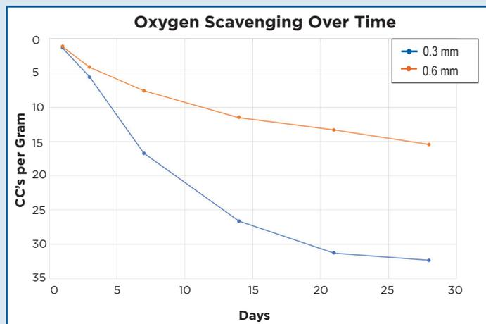
Figure 3: Oxygen Scavenging Performance of Activ-Film™ at Varying Thicknesses
