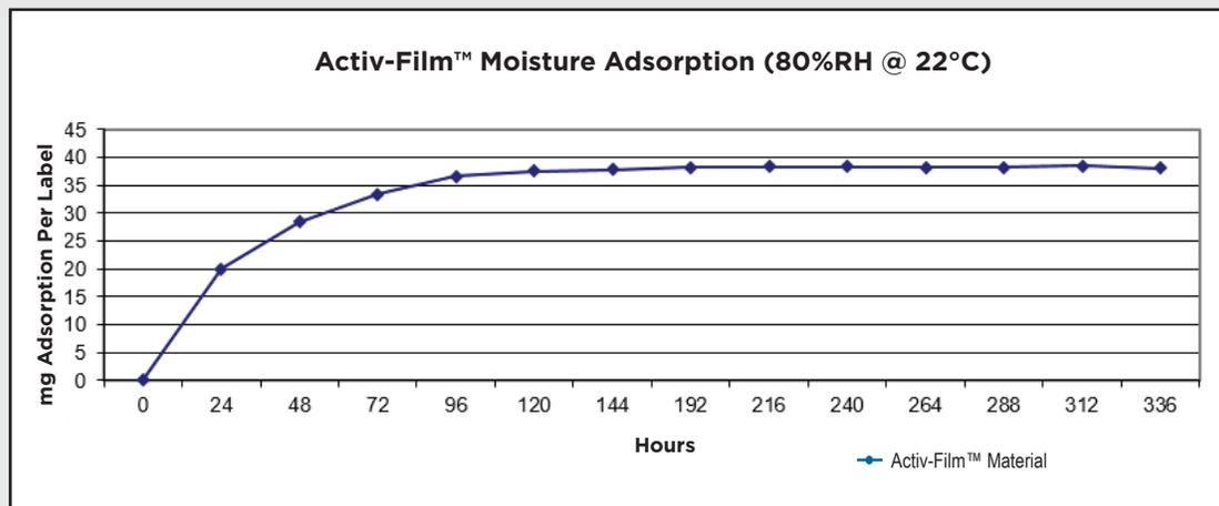
Figure 1: Moisture adsorption of Activ-Film™ at 80% RH and 22°C over time
