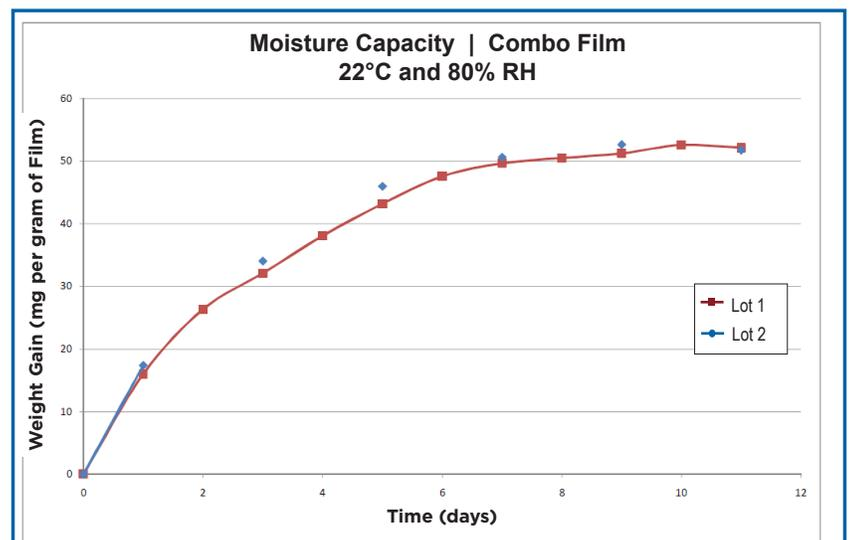
Figure 2: Moisture Adsorption Performance of Combination Activ-Film™ Solution
