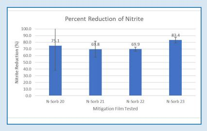
Figure 7: Percent reduction of nitrite in MCC tablets sealed with N-Sorb mitigation films when compared to control sample
