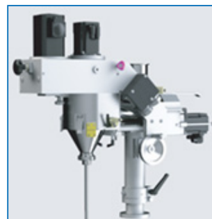
Figure 7: Powder Dosing System
